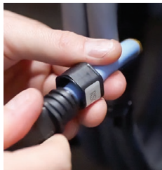
Rogowski coils split to wrap around large conductors
