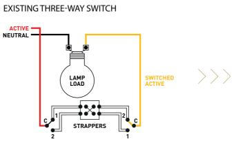
Traditional three-way switching using two rocker switches and one intermediate switch, with strappers between the switches. Rocker switches and intermediate switch are replaced with Diginet LEDsmart<sup>+,</sup> dimmers. The existing strappers are used to connect the dimmers in parallel. No new wiring is required.
