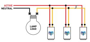
Required wiring for three-way dimming and switching using Diginet LEDsmart<sup>+</sup> dimmers. If more than three dimmers are required, further dimmers are simply wired in parallel.
