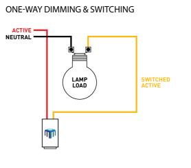
Dimmers without built in switch powered by MultiMate<sup>™</sup> technology connect just like standard two-wire dimmers.
