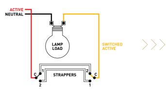
When replacing existing two-way switching with two-way dimming/switching using Diginet LEDsmart<sup>†</sup>™ dimmers, the existing two-way 'strapper' wires can be used. No new wiring is required.
