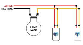
Two-way switching and dimming with Diginet LEDsmart<sup>+</sup>™ dimmers.
