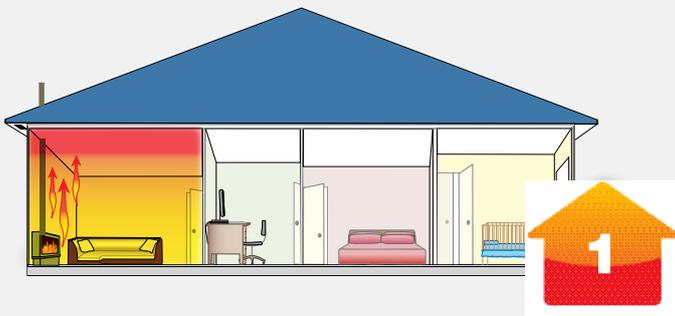
Excess heat from your heat source will rise to ceiling level where it is trapped. This excess heat can reach temperatures of 30-35°C.
